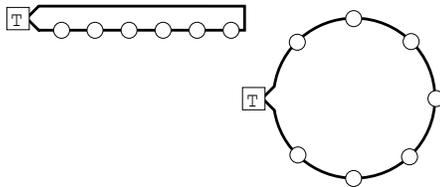
3. Split load installation or multiple cable run: Fixtures run in two or more directions from the transformer. Locating the transformer in the center of the run reduces the effects of voltage drop.
