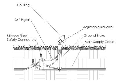
The operating voltage range for this LED luminaire is 9 - 15 volt AC. The Vista electronic driver ensures the LED operates at the intended lumen output while receiving voltage as low as 10.5 volts, and as high as 15 VAC, the U.L. allowed maximum, resulting in a balanced lumen output from the first fixture to the last. Eliminating the dimness issues often attributed to voltage drop.
