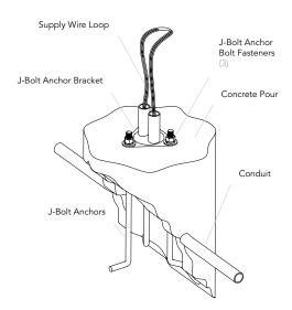
Pour the concrete pad to the top surface of the J-bolt anchor assembly bracket.For best results, ensure that the top surface of concrete is smooth and level.
