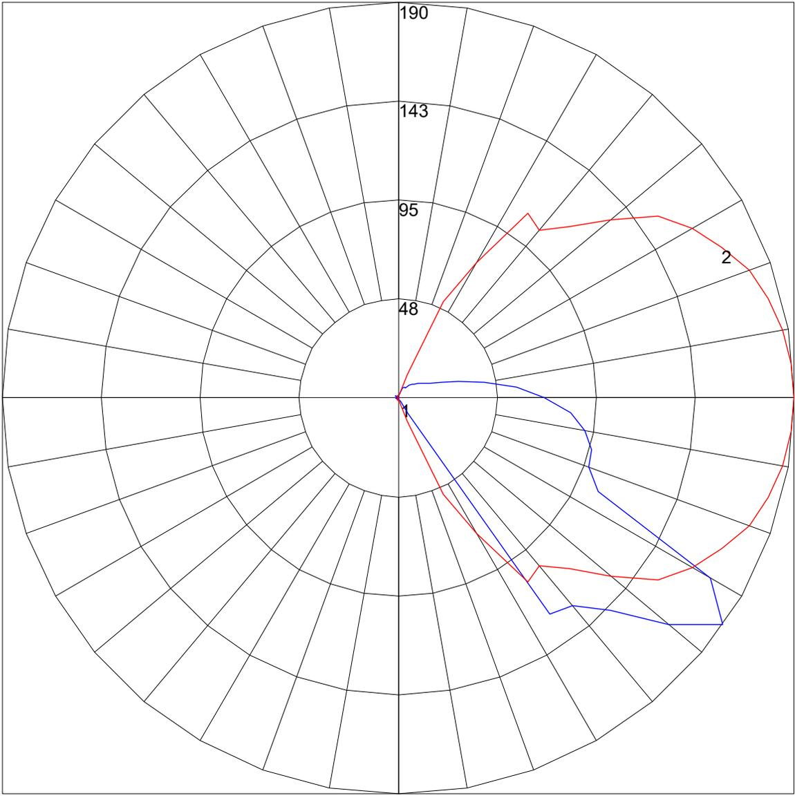
Maximum Candela = 190 Located At Horizontal Angle = 0, Vertical Angle = 55
