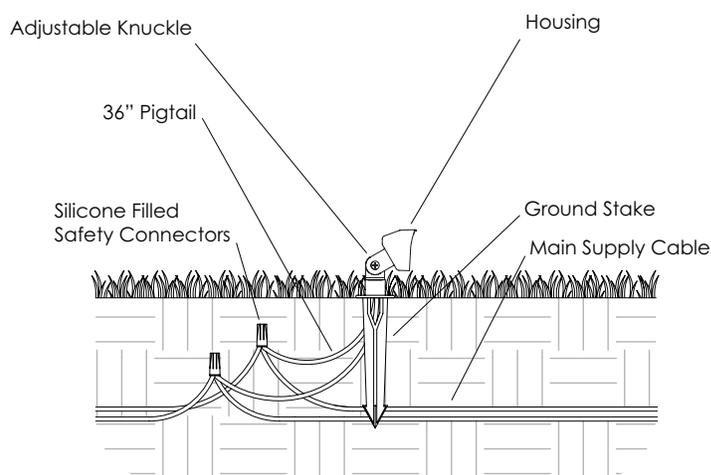
The operating voltage range for this LED luminaire is 9 - 15 volt AC. The Vista electronic driver ensures the LED operates at the intended lumen output while receiving voltage as low as 10.5 volts, and as high as 15 VAC, the U.L. allowed maximum, resulting in a balanced lumen output from the first fixture to the last. Eliminating the dimness issues often attributed to voltage drop.
