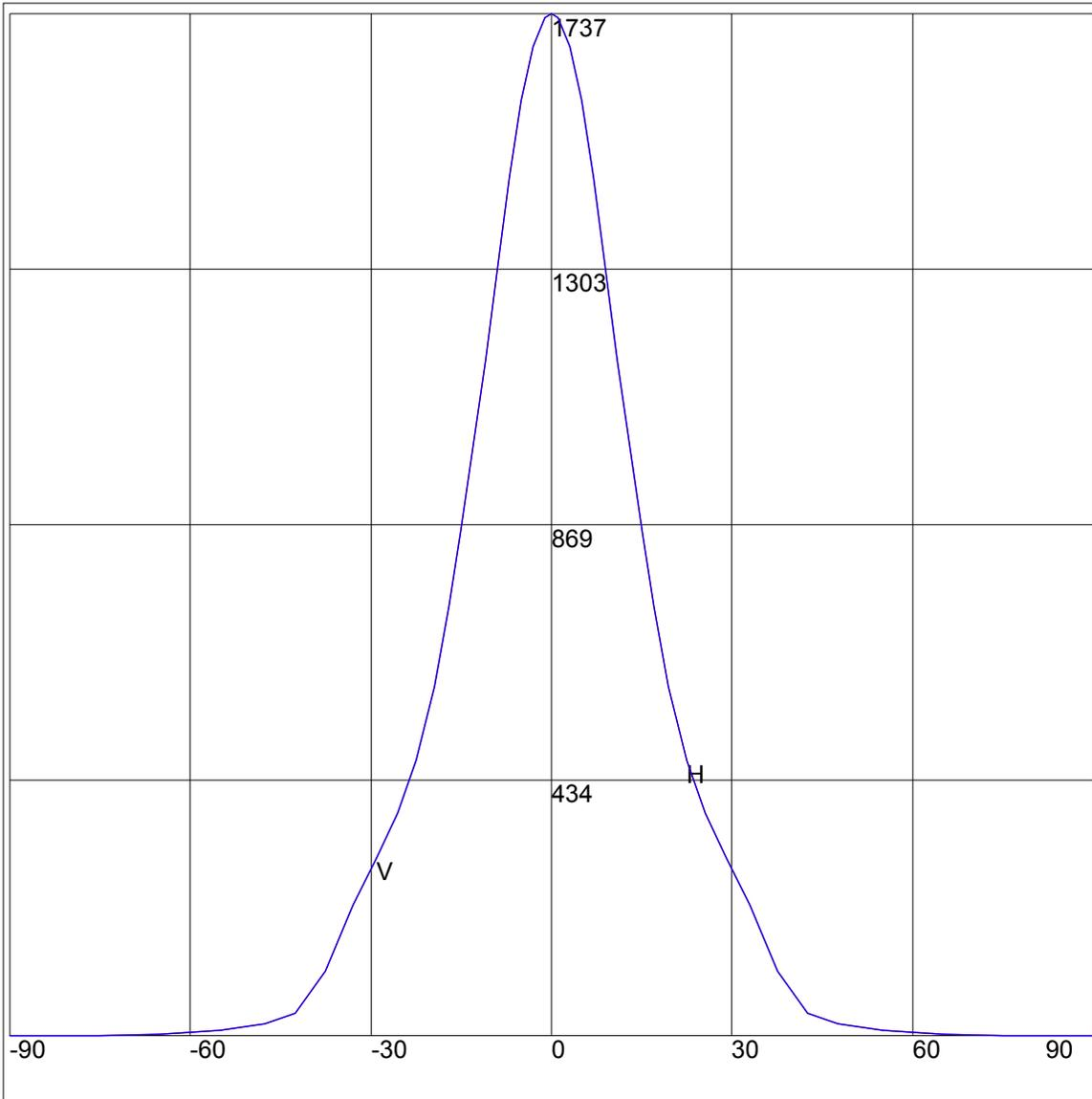
Maximum Candela = 1737 Located At Horizontal Angle = 0, Vertical Angle = 0
