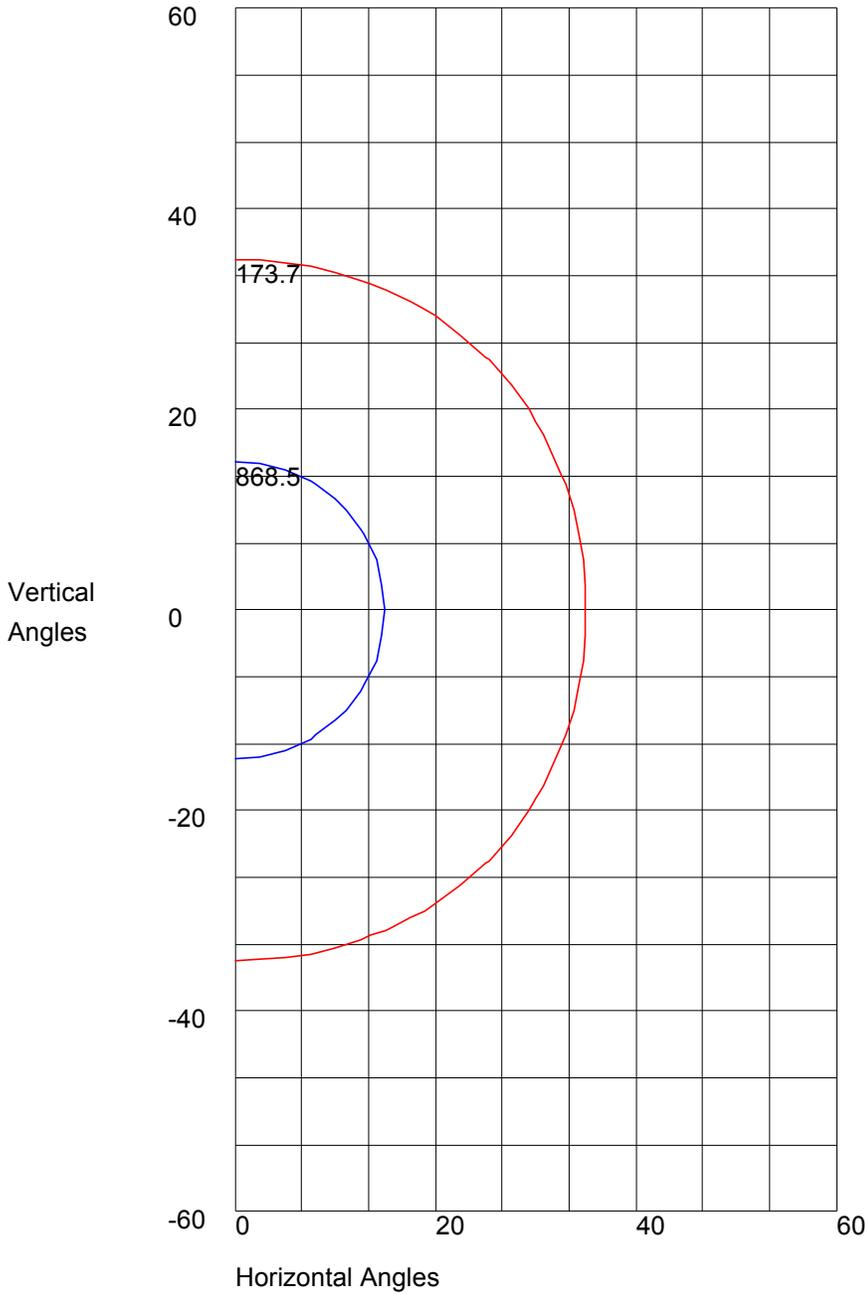
Maximum Candela = 1737 Located At Horizontal Angle = 0, Vertical Angle = 0
