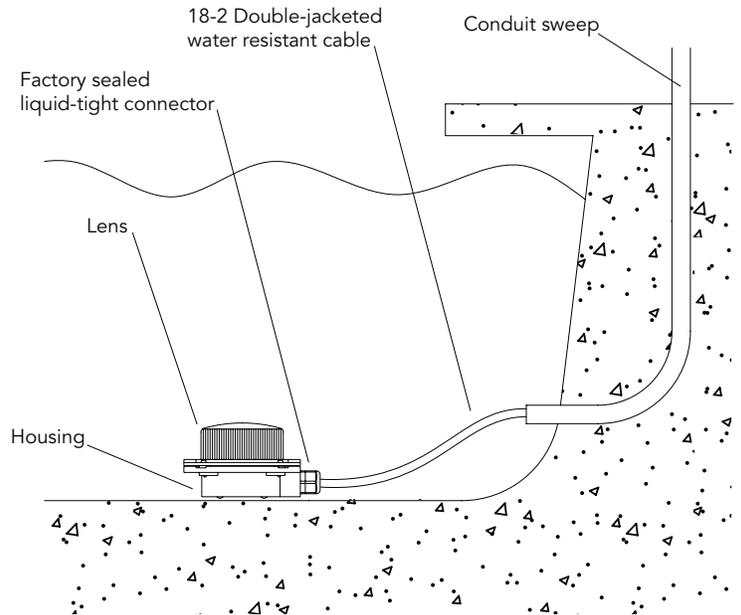
**The operating voltage range for this LED luminaire is 6 - 15 volt AC.** The Vista electronic driver ensures the LED operates at the intended lumen output while receiving voltage as low as 6 volts, and as high as 15 VAC, resulting in a balanced lumen output from the first fixture to the last. Eliminating the dimness issues often attributed to voltage drop.
