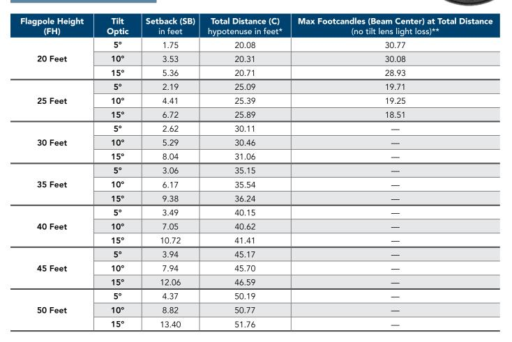
\*FH<sup>2</sup> + SB<sup>2</sup> = C<sup>2</sup> \*\*Footcandle figures are NOT corrected for angle of incidence and have NOT included a 5-6% light loss factor for the tilt optic lens. Calculations are based upon maximum candela measurements for each beam distribution.
